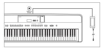
Connect the AC power adaptor to an AC outlet.
